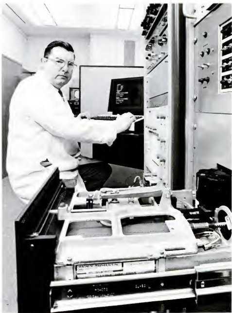
NBS computer standards ensure that Federal agency computer users will be able to purchase equipment competitively from independent suppliers. In the Bureau's magnetic media laboratory, electronic engineer William Truitt calibrates flexible disks for use as Standard Reference Materials.
