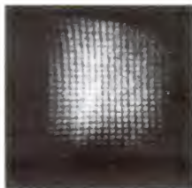
An NBS research team led by physicist Masao Kuriyama has developed a new device and technique for nondestructive evaluation that magnifies x-ray images on a real-time basis with significantly improved image resolution. Shown above is a radiograph of a lead-copper casting taken with the x-ray magnifier.
