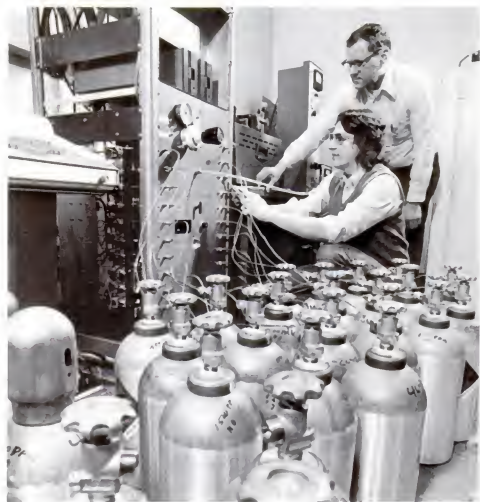
Engineering technician James Suddueth (standing) and Research Associate Robert Miller prepare to analyze gaseous Standard Reference Materials using a computer-operated gas analysis system developed at NBS. At right, engine exhaust from a new automobile is measured at an EPA facility using NBS-recommended techniques.
